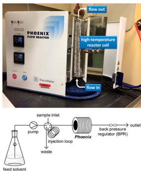
Figure 1. Schematic of the high-temperature Phoenix flow reactor.
